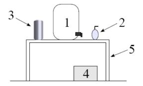
The water container (**labeled #1**) must be designed with a spigot that allows the user a continuous flow of water to wash hands freely without continuously depressing the spigot or tilting the container. Other types of water containers may be used but must be approved in advance by the health authority.
